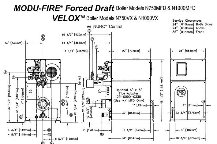
MODU-FIRE® FD boilers require Category II (condensing-negative pressure) or Category IV (condensing-positive pressure) venting and VELOX™ boilers require Category I (non-condensing) venting as defined in ANSI Z223.1/NFPA 54/CSA-B.149 Latest Edition. Horsco Industrial, Potterson-Kelley reserves the right to make changes at any time mithout notification.
