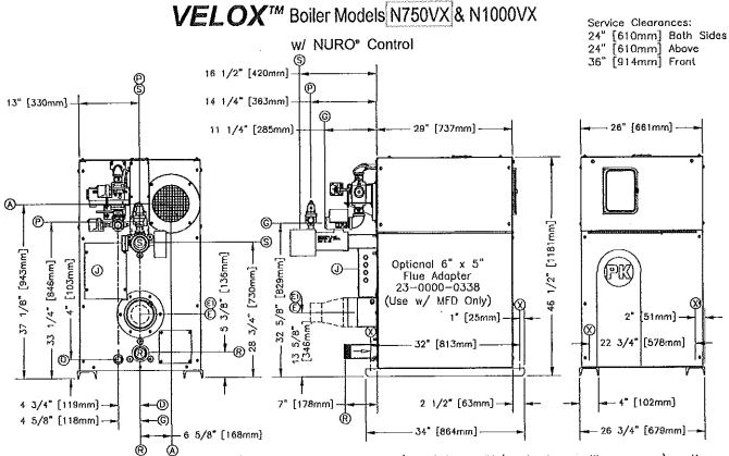
MODU-FIRE® FD boilers require Category II (condensing-negative pressure) or Category IV (condensing-positive pressure) venting and VELOX™ boilers require Category I (non-condensing) venting as defined in ANSI Z223.1/NFPA 54/CSA-B.149 Latest Edition. Horseo Industrial, Patterson-Kelley reserves the right to make changes at any time without notification.
